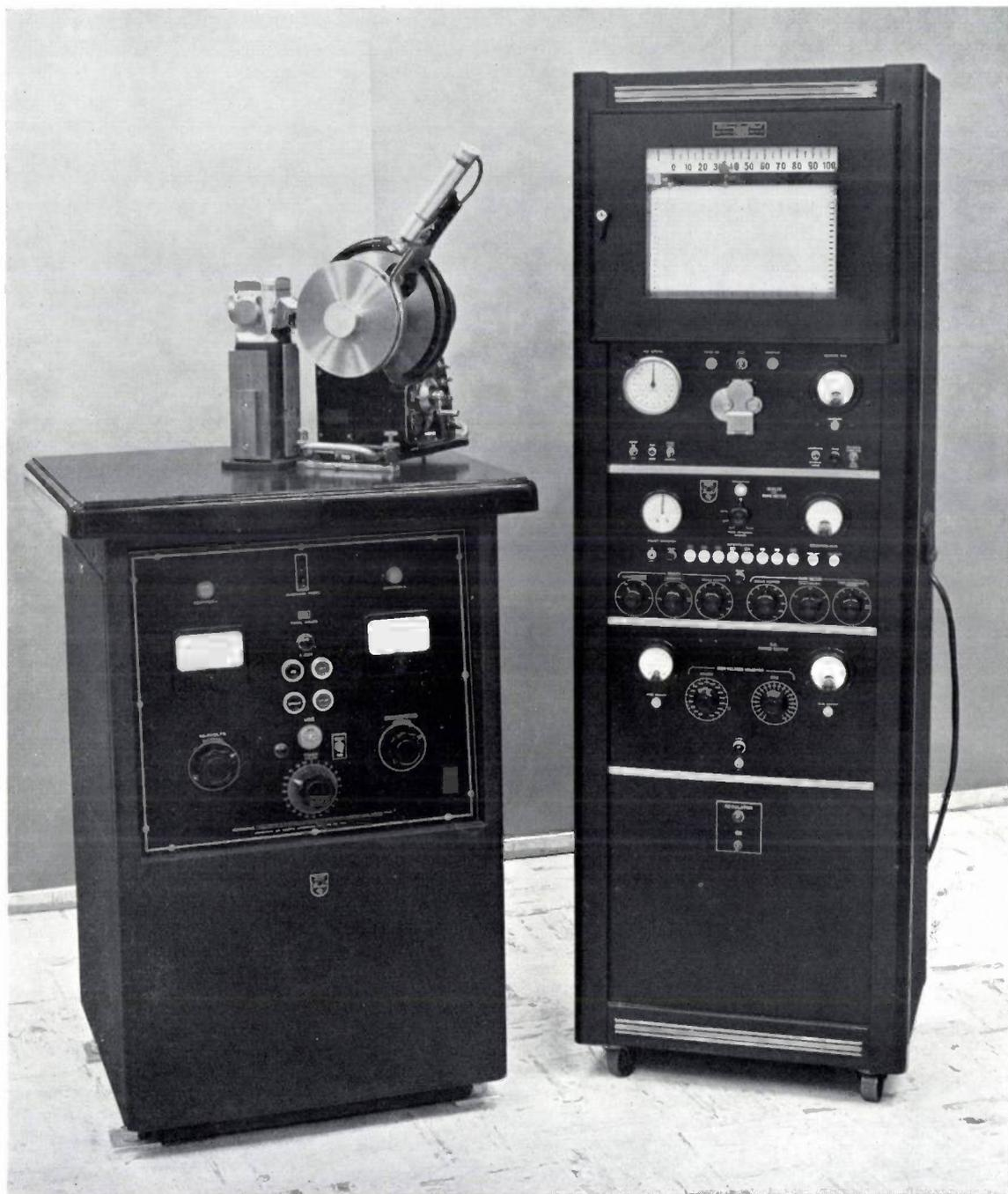
Fig. 2. The "Norelco" Geiger counter diffractometer consists of three independent parts: a basic diffraction unit (X-ray tube with high voltage generator and controls, at left), the high angle precision Geiger counter goniometer placed on top of it, and an electronic circuit rack with automatic 10" strip chart recorder (at right).
