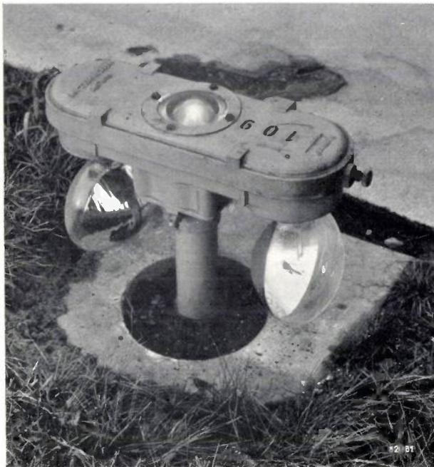
Fig. 15. Elevated runway light, as employed on a number of airfields in the Netherlands. Two special lamps, similar to that shown in fig. 12 but rated at only 100 W, are suspended back to back to shine in the two landing directions of the runway. The cover contains an omni-directional light.
