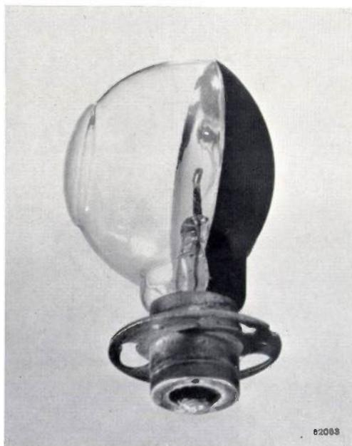
Fig. 19. Special 35-W lamp employed in a flush runway light. Part of the bulb, in the form of an ellipsoid of revolution, is silvered on the inside. Height of lamp:  $2\frac{1}{2}$ ".
