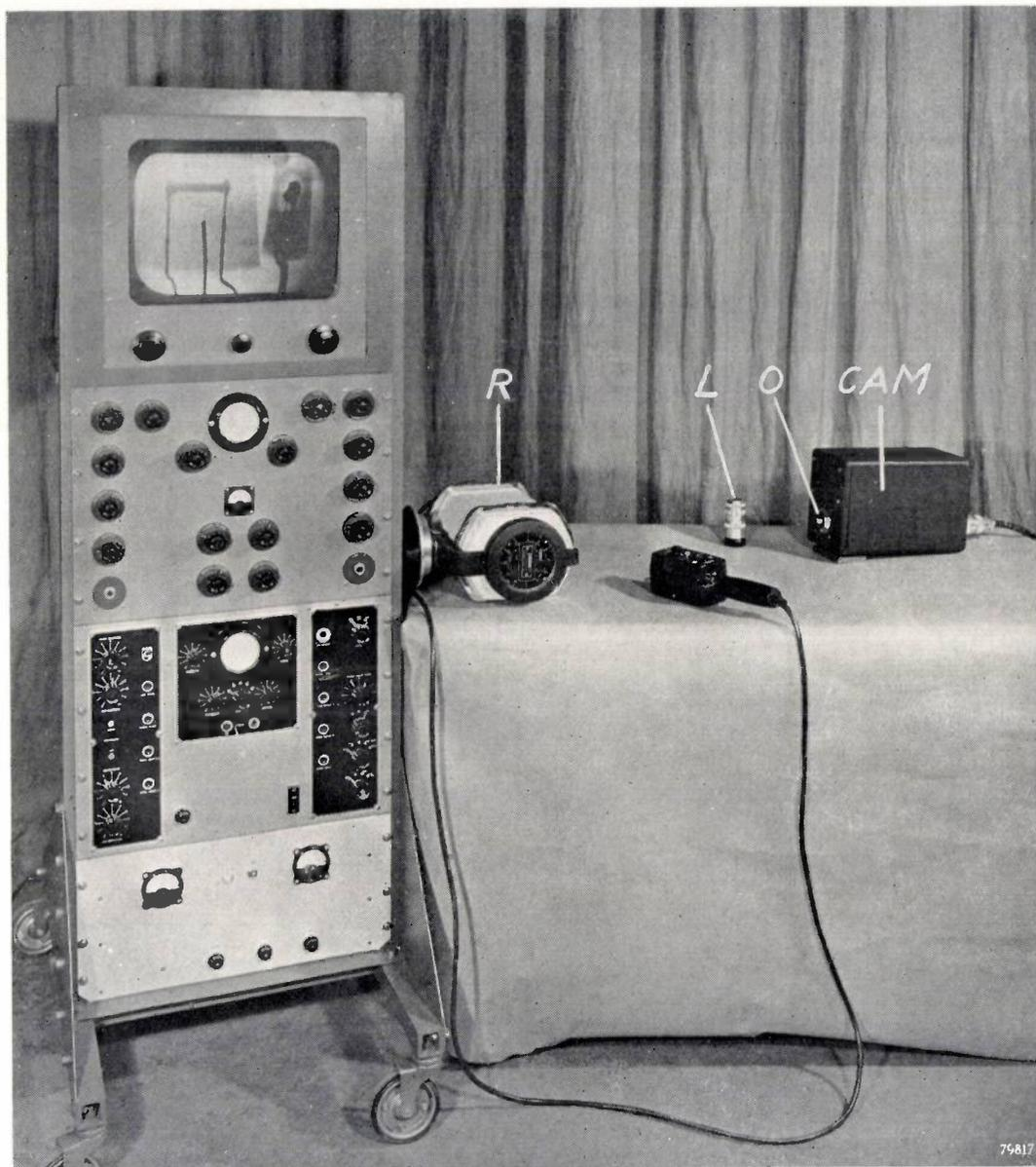
Fig. 2. Set-up for making the photograph shown in fig. 1b. CAM television camera with the new camera tube. Lens (*L*) has been removed and the object to be irradiated (*O*, in this case two transistors) has been placed directly in front of the tube. *R* is the X-ray tube ("Practix"). On the screen of the picture tube, to the left, the greatly enlarged X-ray shadow image of the two transistors is visible.
