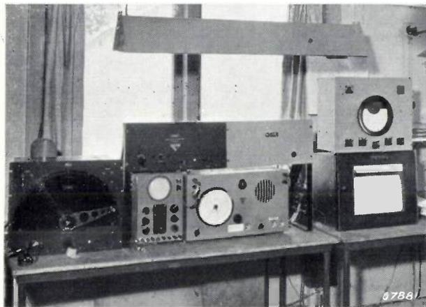
Fig. 10. Photograph of the ground-station receiving equipment as installed in the Royal Dutch Meteorological Institute. The F.M. receiver is seen at the centre, and the recording meter on the right. At the extreme left is the calibrating equipment which supplies a constant comparison-frequency. Calibration is preferably effected with the aid of a cathode-ray oscillograph.
